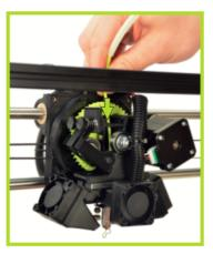
To lock the filament in place, compress the springs with the idler retainer and rotate the hinged idler clockwise into an upright position. Lock the hinged idler into place by sliding the idler retainer back down into the locked position. Then tighten the retainer screws if you loosen them previously.
