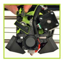
When the nozzle head is up to temperature you can insert the filament into the feed hole (see the pictures below). If there is filament that you wish to remove, you simply pull the filament out of the feed hole and then insert your desired filament. Note, filament should not be removed unless the nozzle head is hot. Push the filament into the feed hole until filament begins to extrude out of the nozzle head. This may require a firm push.
